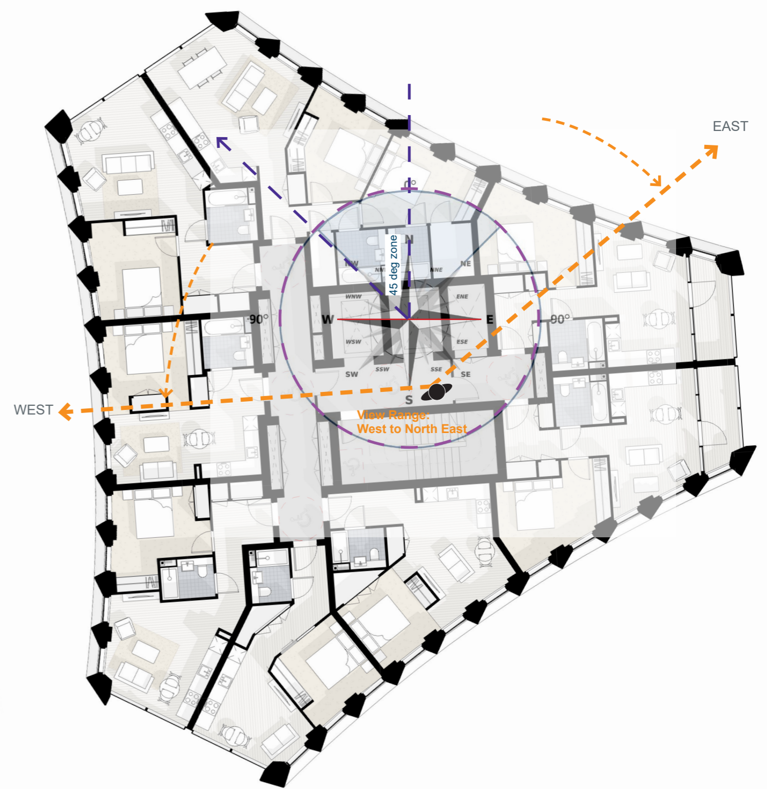
Block A - Tower - Unit Orientation
